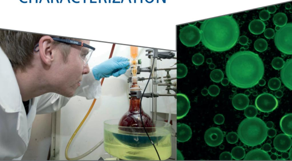
The Keylab combines the expertise and equipment for the synthesis of functional polymers and their characterization. Reactors ranging from 0.05 – 10 L are available for polymer synthesis from the gram to the kilogram scale.
